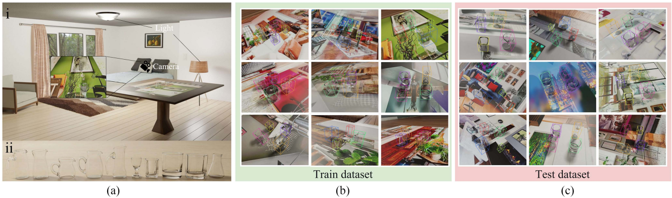
Fig. 2. (a) Dataset generation scenarios. (i) Scene setup for generating the transparent object synthetic dataset using Blender. (ii) Transparent object CAD models, #01 to #10 from left to right. (b) Train dataset in Trans6D-32 K. (c) Test dataset in Trans6D-32 K.
